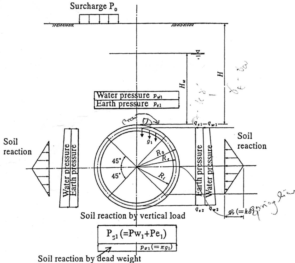
$$\begin{aligned}\text{Vertical Pressure} &= \text{Soil Pressure} + \text{Water Pressure} + \text{Pressure from Surcharge Load} \\ &= (\gamma_{dry}H) + (\gamma_w H) + (P_o \times \text{Disdribution Factor})\end{aligned}$$
